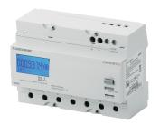
The COUNTIS E3x is a modular energy meter displaying the energy and power consumed (kWh and kW) directly on its backlit LCD display. It is designed for three-phase load metering and is used for direct connections of up to 100 A. COUNTIS E32, E34 and E36 are also MID-certified.
